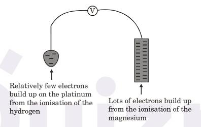
There is a major difference between the charge on the two electrodes - a potential difference which can be measured with a voltmeter. The voltage measured would be 2.37 volts and the voltmeter would show the magnesium as the negative electrode and the hydrogen electrode as being positive.
