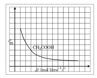
The very large increase at infinite dilution is because the ionization increases and so the number of ions in solution increases.
