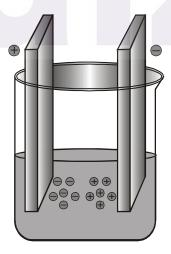
The negative ion is pulled to the negative pole because it is surrounded by positive charges and vice versa.
