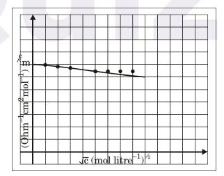
This is because at higher concentration there is greater inter ionic attraction which retards the motion of the ions as conductance falls  $\wedge_m^c$  and  $\wedge_m^\infty$  is that conductance at infinite dilution where the ions are far apart and there is no inter-ionic attraction. This can be obtained by extrapolation of the graph to zero concentration.
