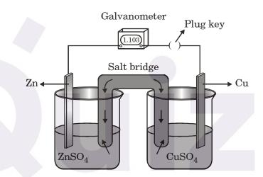
The two aqueous solutions are interlinked through a salt bridge which is an inverted 'u' tube which is filled with saturated semi solid paste of Agar Agar saturated in KCl or  $KNO_3$  solution [Agar agar is a carbohydrate which forms a jelly like substance when dissolved in hot water]
