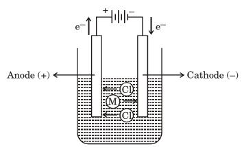
Thus, electrolysis is a process of chemical decomposition of the electrolyte by the passage of electric current. It is carried out in a cell called **electrolytic cell**.
