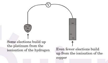
There is less difference between the electrical charges on the two electrodes, so the voltage measured will be less. This time it is only 0.34 volts.
